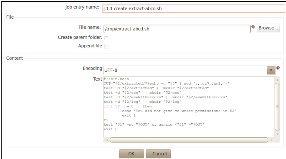
Figure J.1.1a Settings of the “Write to file” step
