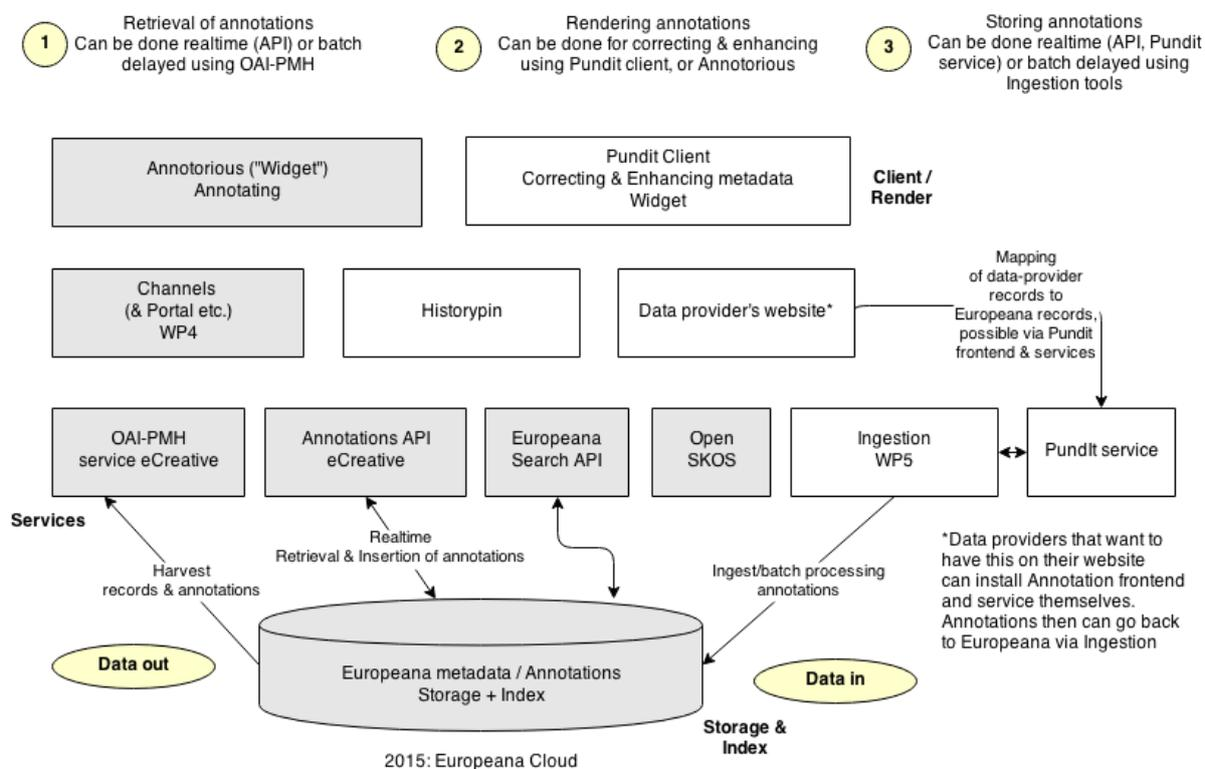
This is a draft sketch for the data flow/eSounds architecture based on D2.1 & D2.2. Final (technical) architecture & components to be created after D2.2. Grey-coloured are Europeana current and/or future plans. Annotations API & OAI-PMH to be integrated and ready estimated Q1 2015.
